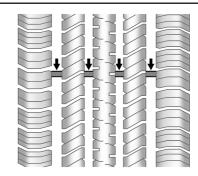
Treadwear indicators are one way to tell when it is time for new tires. Treadwear indicators appear when the tires have only 1.6 mm (1/16 in) or less of tread remaining. See *Tire Inspection* ⇒ 343 and *Tire Rotation* ⇒ 343.
