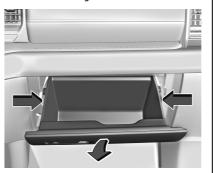
Press the sides of the glove box door inward and rotate the door downward to remove.
