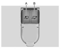
If equipped with the fifth-wheel/gooseneck trailer package, the harness connector is mounted on the inside of the pickup bed behind the rear wheel.
