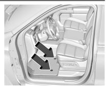
Reinstall by lining up the floor mat/liner retainer openings over the carpet retainers and snapping into position.
