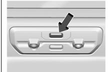
The MultifFex (Chevrolet)/MultiPro (GMC) inner tailgate may be equipped with an enable/disable feature to prevent the inner tailgate from being opened when a hitch or other equipment is installed that could damage the inner tailgate.
