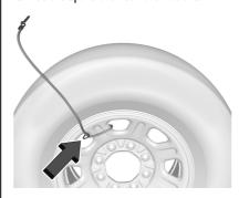
If equipped with a spare tire cable remove the cable from the spare tire by passing the clip through the looped end of the cable.
