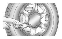
If the wheel has a smooth center cap, concealing access to the wheel nuts, place the chisel end of the wheel wrench in the slot on the wheel, and gently pry it out.
