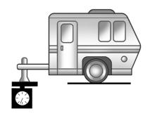
Do not exceed a maximum trailer tongue weight of 567 kg (1,250 lb) for a conventional trailer hitch.
