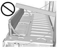
Do not place a load on top of the step when using it as a load stop.
